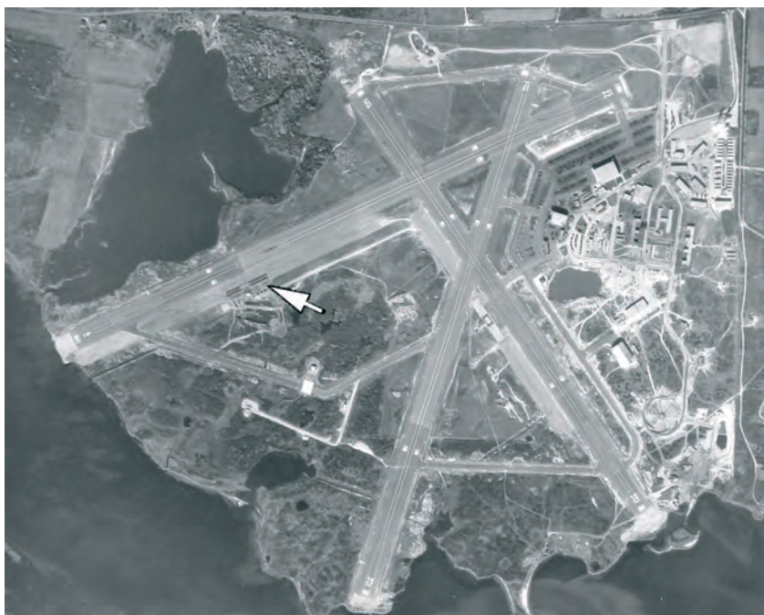
Aerial view of Charlestown Naval Auxiliary Air Field, 1945. The structure adjacent to Runway 22 (arrow) may be the wood deck built for catapult and carrier-landing practice. (National Archives)
