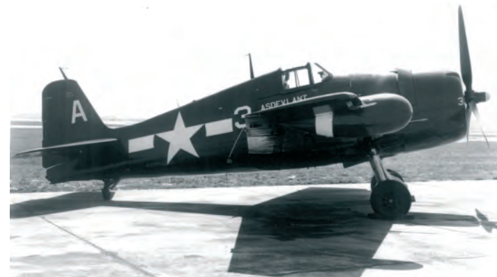
The Navy experimented with Hellcats equipped with radar and searchlights for anti-submarine duty. (New England Air Museum)
