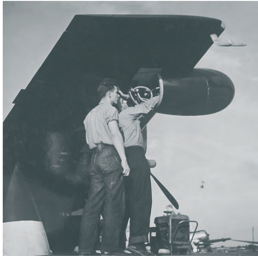
Above: CASU-27 technicians service an APS-6 radar unit aboard a Hellcat night fighter at Charlestown during World War II. The unit had a rapidly rotating antenna that required frequent attention. The rear fairing of the radar nacelle can be seen on the ground at the left. (National Archives)
