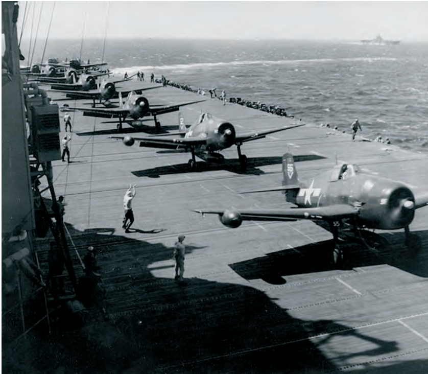
F6F Hellcats lined up for take-off aboard the carrier Ticonderoga during World War II. The first two planes are radar-equipped night-fighters. (National Archives)
